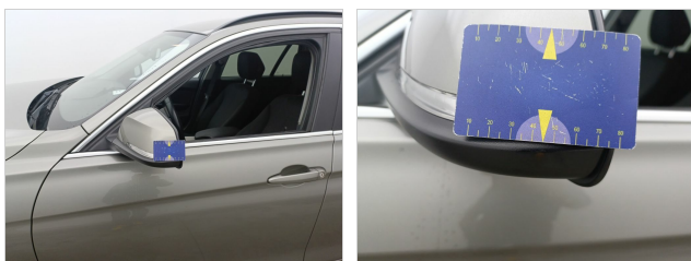
Side View Mirror Left // Plastic Repair: E - Scratch
