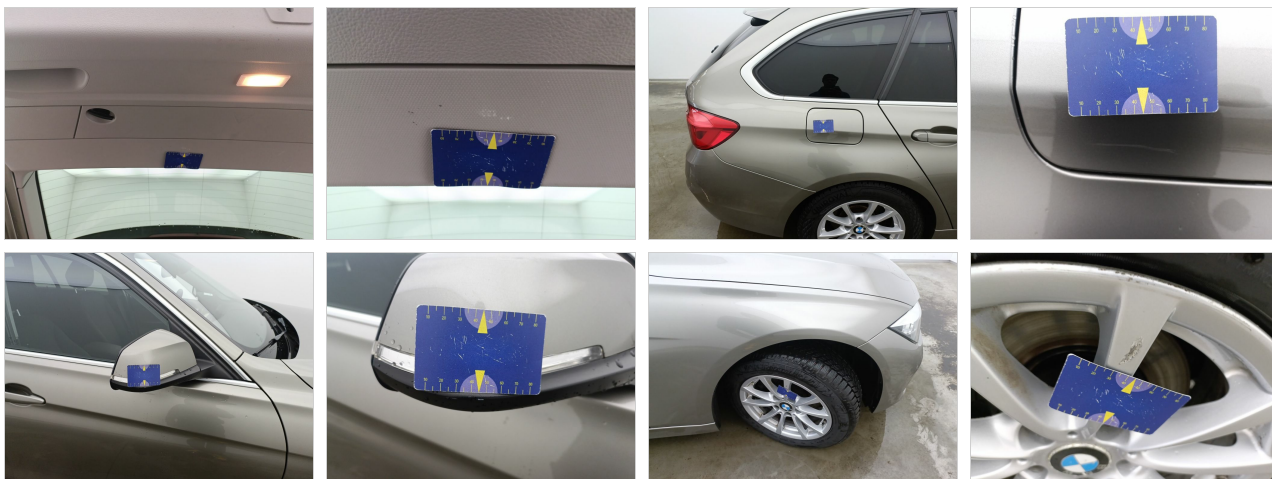
Damage within Renta-norm
