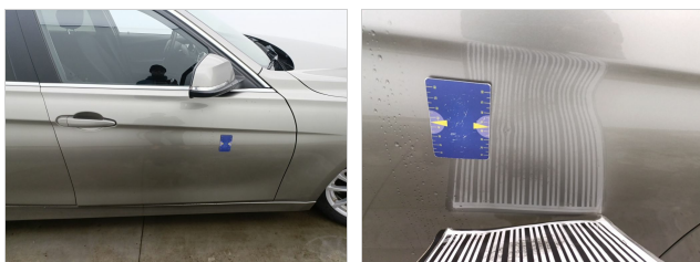
Door Front Right // Smart Repair Small: AA - Scratch +Dent
